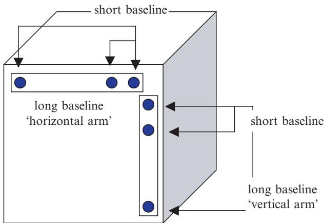
**Fig. 3.** Possible arrangement of long and short baseline interferometer antenna elements on the satellite side panels.
